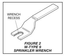
**Step 2.** Tighten the sprinkler into the sprinkler fitting using only the W-Type 9 Sprinkler Wrench as shown in Figure 2, except that an 8 in. or 10 in. adjustable crescent wrench is to be used for wax coated sprinklers. With reference to Figure 1, the W-Type 9 Sprinkler Wrench is to be applied to the wrench area, or as applicable, an adjustable wrench is to be applied to the wrenching flanges.
