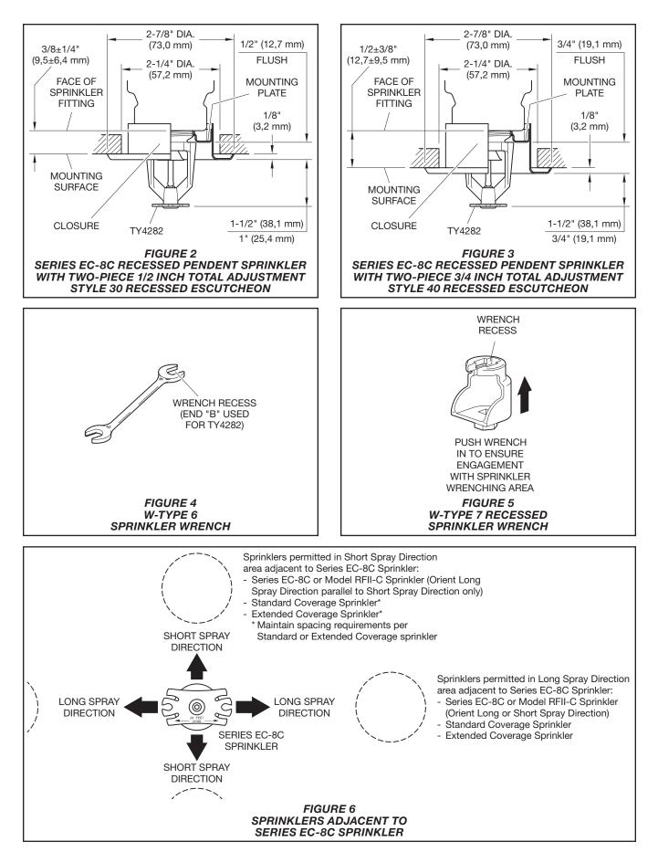
Do not attempt to compensate for insufficient adjustment of an escutcheon plate by under-or over-tightening the sprinkler. Re-adjust the position of the sprinkler fitting to suit.
