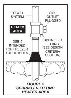
maximum torque of 20 ft-lb to 30 ft-lb (26,8 N·m to 40,2 N·m). Higher levels of torque may distort the sprinkler Inlet with consequent leakage or impairment of the sprinkler.
