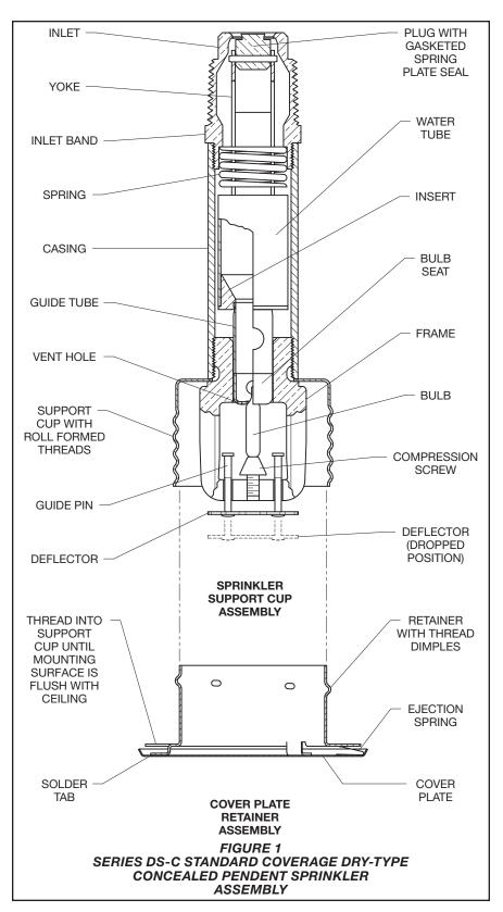
The compressed spring is then able to expand and push the water tube as well as the guide tube outward. This action simultaneously pulls inward on the yoke, withdrawing the plug with gasketed spring plate seal, from the inlet, allowing the sprinkler to activate and flow water.
