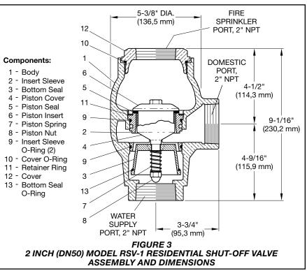
When using the 2 inch RSV-1, the maximum flow rate through the Internal By-Pass Restriction, when the Model RSV-1 Valve is in the operated position, is no greater than 1.5 GPM (5,7 LPM) for a typical residual (flowing) pressure of 40 psi (2,8 bar) at the inlet. Conse-
