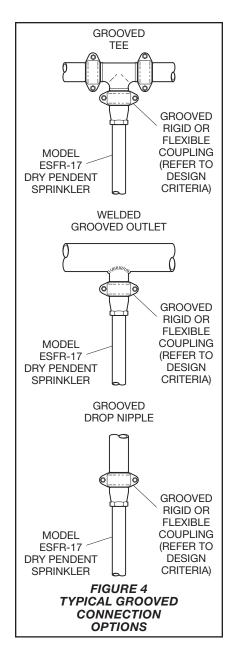
When using tees, use of the Figure 219 GRINNELL Grooved Ductile Iron Cast Fittings (Refer to TFP1810) is recommended.
