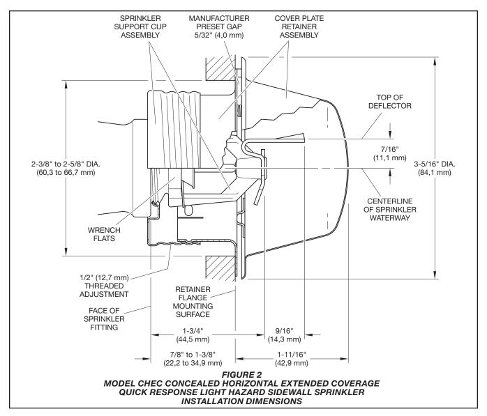
specified in the current NFPA 13 for extended coverage sidewall sprinklers.
