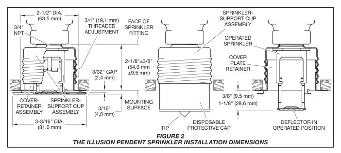
Do not attempt to compensate for insufficient adjustment in the sprinkler assembly by under-or over-tightening the sprinkler/support cup assembly. Readjust the position of the sprinkler fitting to suit.
