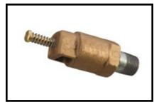
Upon system operation and flow of water through the alarm trim to the alarm devices, the Model AD-1 Automatic Drain Valve automatically closes upon increasing flow between 2 to 10 GPM (8 to 38 LPM), which will then divert waterflow pressure to the alarm devices such as a pressure alarm switch or water motor alarm. When the Model AD-1 Automatic Drain Valve is closed and pressurized, a small leakage past the ball seat is normal.
