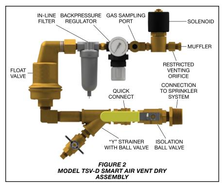
Step 5. Close the isolation ball valve and allow device to depressurize through restricted venting orifice to pressure setting. Make adjustment to pressure setting using the knob, then open the isolation ball valve to pressurize device and close the isolation ball valve again to check pressure setting. Repeat process until desired pressure setting is achieved.
