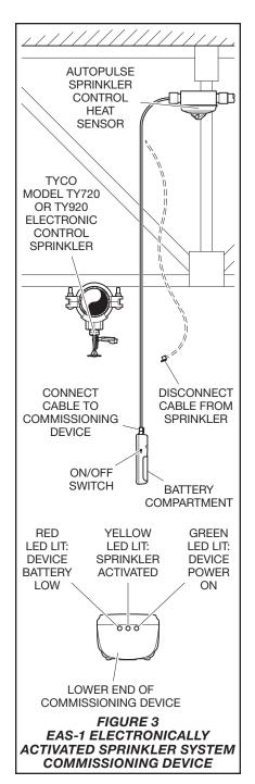
**Step 8.** Confirm the Yellow LED is lit on the EAS-1 Commissioning Devices connected to at least three of the four remaining sprinkler control heat sensors.
